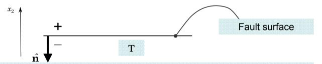
Shear traction that a particle loacted on the "-" side exercised on particle located in the "+" side
