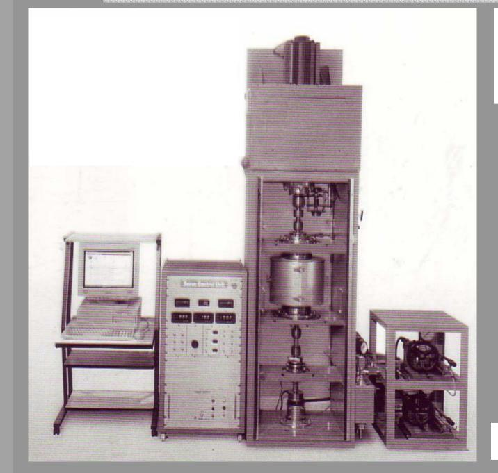
$u_{tot}$  = infinite  $v = 0.1 \ \mu m/s - 10 \ m/s$  $\sigma_n^{eff} < 20 \ MPa$
