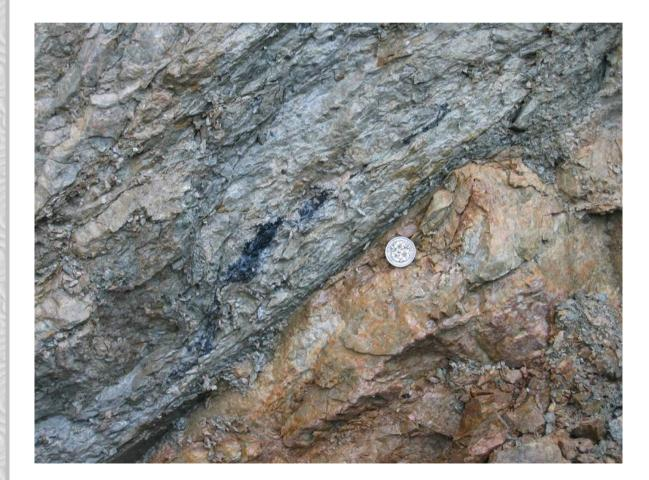
MTL: Fractured mylonite, cataclasite and gouge
